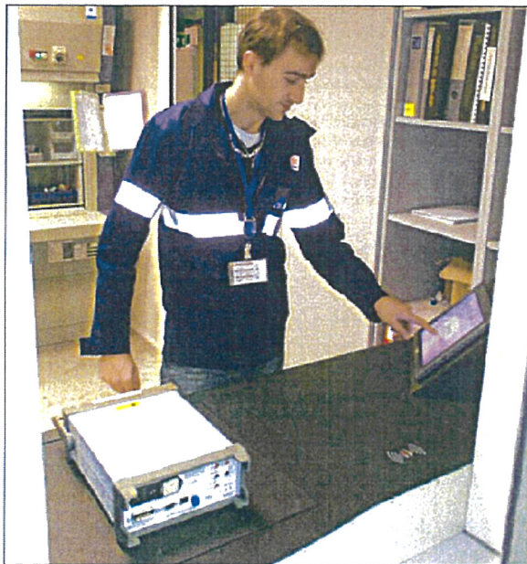
Nexess' smart counter system consists of a touchscreen, an RFID reader and a weight scale.
